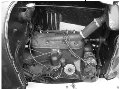
All the important gizmos are on the off side of the Morris Cowley engine unlike the Calthorpe
